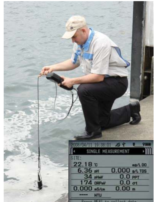
Water quality monitor displays 11 parameters simultaneously
